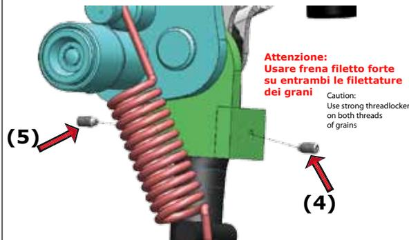
*Insert the anti-theft by helping and manually centering the block graft in the mobile plate hole, first tighten the grub screw (5) of the movable plate until the plate clearance is eliminated without forcing and then the other (4) until making everything the assembly integral with the stand. Always use on the threads a substance which brakes a strong thread like Loctite. Check by inserting and unplugging several times the system is working properly.*
